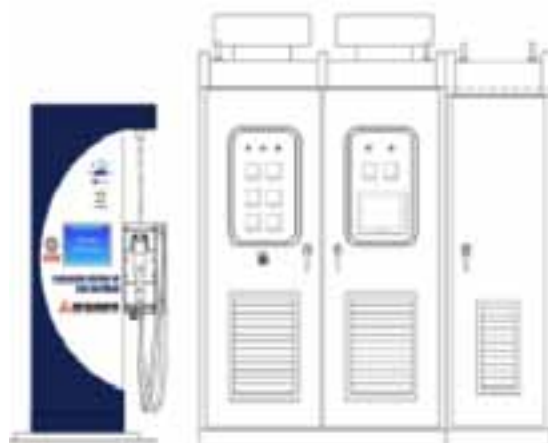
Figure 3-5 Battery combined charging station
