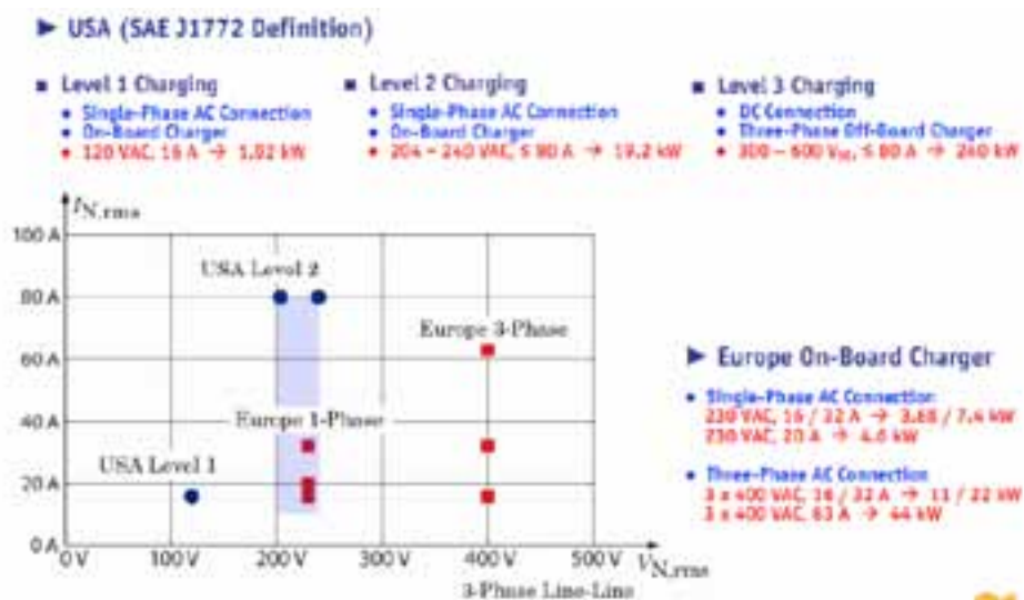
Figure 1-1 Various AC charging specifications
